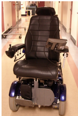
Figure 1. Research wheelchair instrumented with the Virtual Seating Coach.
